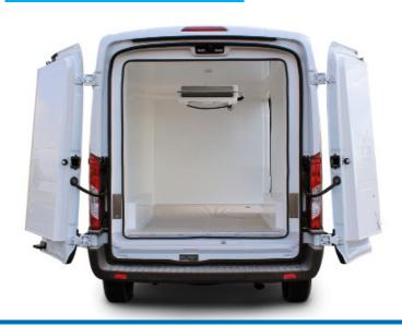
Fully Integrated & Climate Controlled Cargo Insulation System
